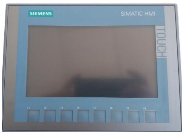
Figura 3.34. HMI Siemens Simatic KTP700 Basic [56].
