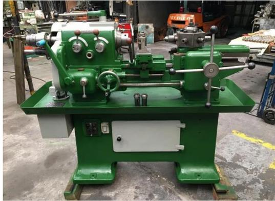
**Figura 2. 8.** Torno revolver
