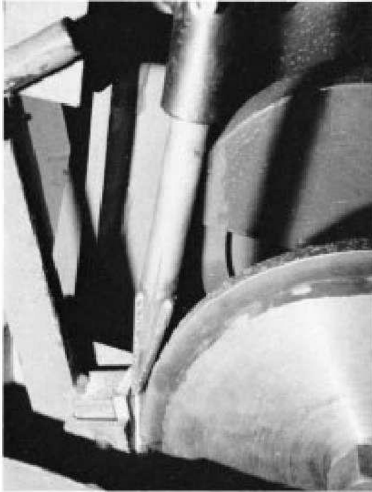
FIG. 8 Position of Sand Nozzle
