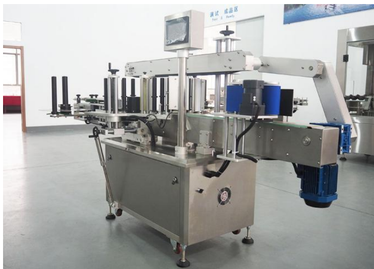
Figura3.11: Etiquetadora Front And Back Panel Labels
