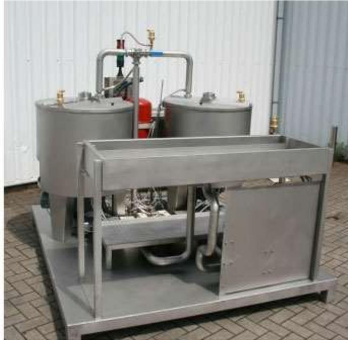
**Figura 3.25.** Máquina Industrial Fundidora de Chocolate.
