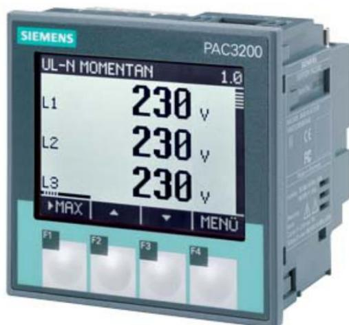
SETRON PAC3200; LCD; 96X96MM POWER MONITORING DEVICE PANEL MOUNT TYPE FOR MEASUREMENT OF ELECTR. VALUES VAUX: 110-340VDC / 95-240VAC VIN: MAX.690/400V; 45-65HZ AMPIN: X/1A OR X/5A AC COMPRESSION TYPE TERMINALS
