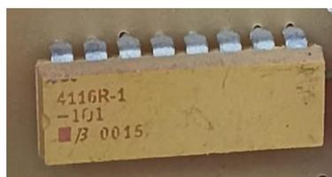
Figura 6. Resistor 411GR-1-101
