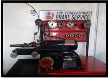
A photograph of a red Ammco 7000 brake drum lathe. The machine has a black motor and a red frame. A sign on the front reads "THE PROFESSIONAL AMMCO BRAKE SERVICE". |
