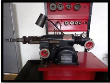
A photograph of a red Ammco 3000 disc lathe. The machine has a black motor and a red frame. It is designed for grinding brake discs.                               |
