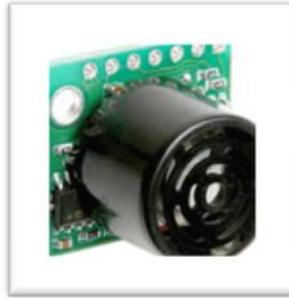
Fig 1.10 Sensor Max Sonar EZ1
