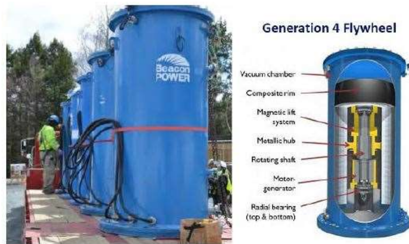
Figura 8. 6.- Volante de inercia FES (FLYWHEEL ENERGY STORAGE) [16]
