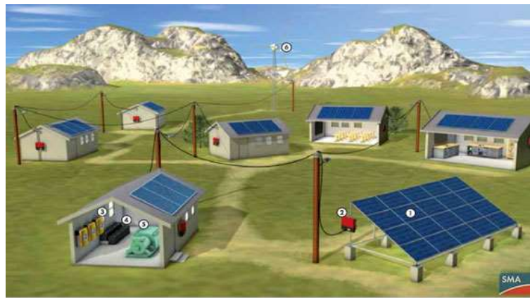
Components: 1. PV array, 2. SUNNY BOY, 3. SUNNY ISLAND, 4. Batteries, 5. Diesel generator, 6. Wind turbine system
