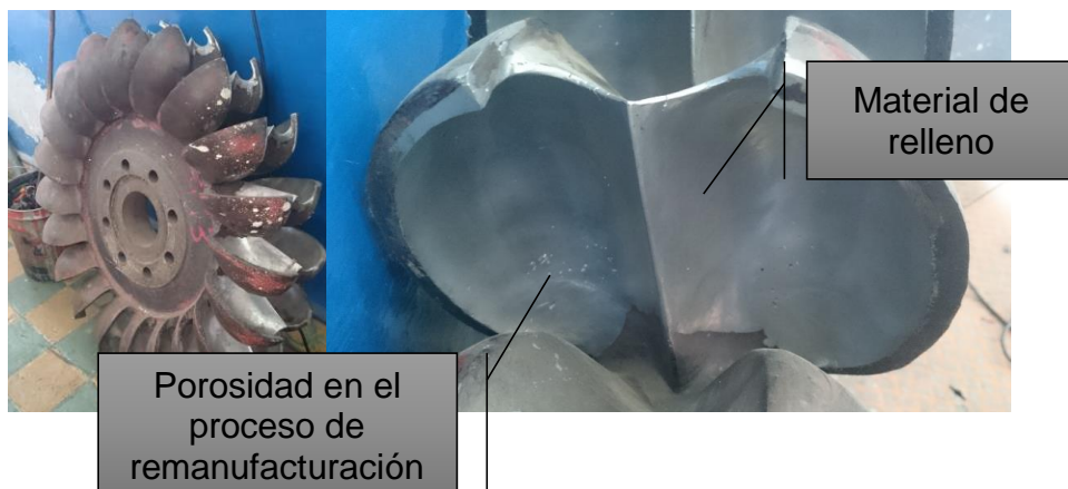
Turbina Pelton central Bell – Kriens 2000 CV / 900 rpm remanufacturada.
