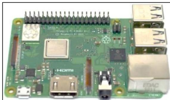
**Figura 9.** Tarjeta Raspberry Pi 3 B+
