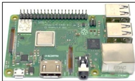
**Figura 5.20.** Tarjeta Raspberry Pi 3 B+
