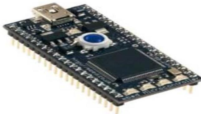
**Figura 5.2 Tarjeta mbed NXP LPC1768 prototyping board**
