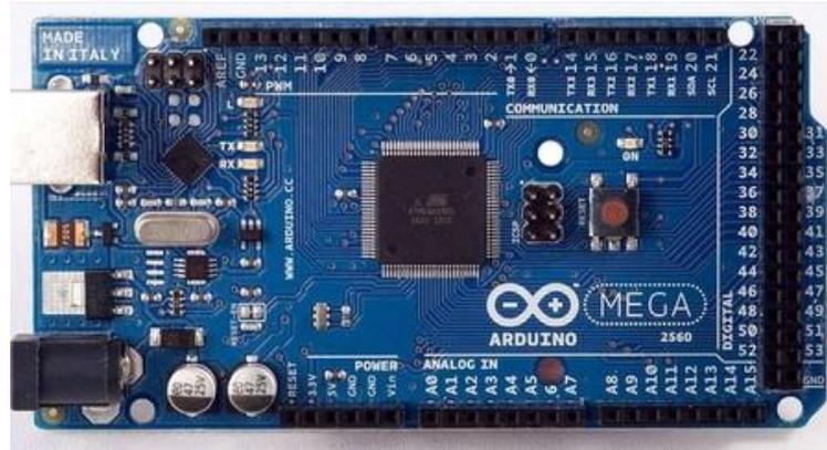
**Figura 3.5.** Arduino Mega [8]
