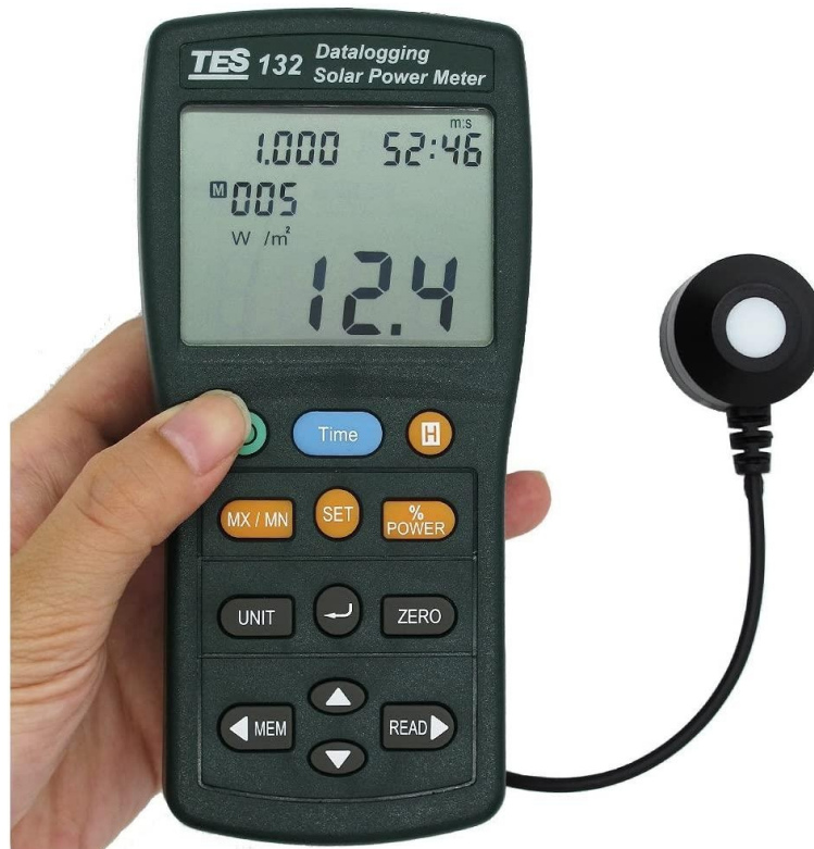
Fig. 6. Datalogging Solar Power meter TES-132
