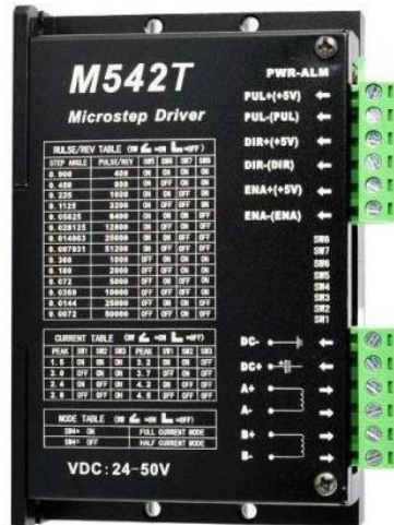
Figura 4.16. Control Driver M542T. [30]
