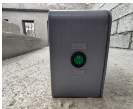
a) Interruptor ON-OFF
