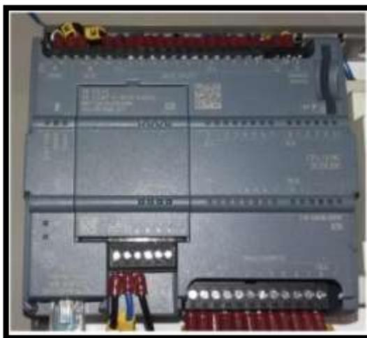
**Figura 4.1** PLC SIEMENS CPU 1214C AC/AC/AC y módulo SIGNAL BOARD SB 1224 [27]
