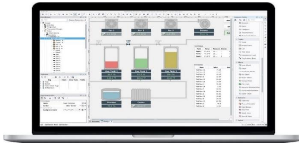
Figura 3.14 Software SCADA Ignition
