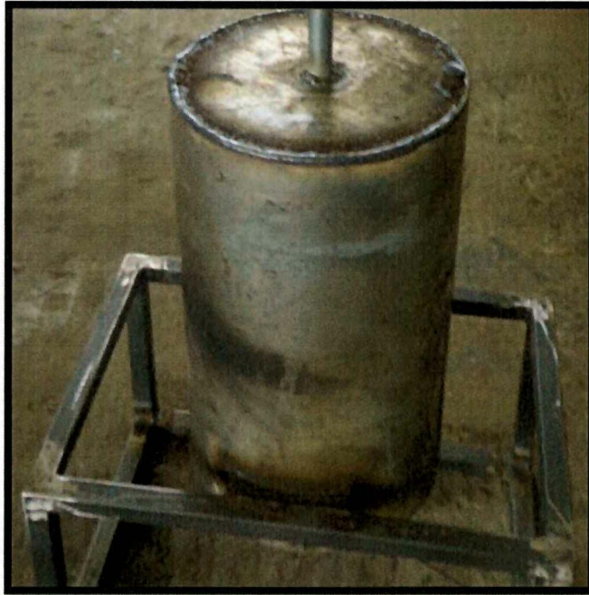
FIGURA 3. 5 REACTOR (CILINDRO PRINCIPAL)
